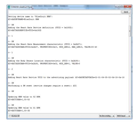
If you open up an application on your mobile device or laptop that support the standard <u>Heart Rate Monitor Service</u> (https://adafru.it/f4l), you should be able to see the heart rate being updated in sync with the changes seen in the Serial Monitor:
