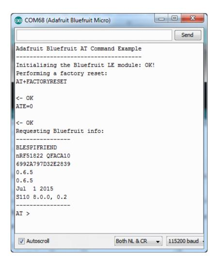
This sketch starts by doing a factory reset, then querying the BLE radio for details. These details will be useful if you are debugging the radio. If you see the information as above, you're working! (Note that the dates and version numbers may vary)
