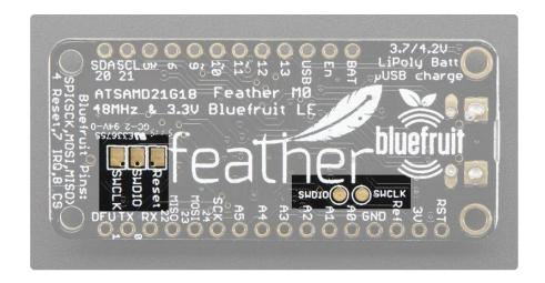
The round pads on the right are for the ATSAMD21G18 (main processor). The rectangular pads to the left are for the nrf51822 inside the BLE module.
