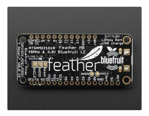
The Feather MO Bluefruit uses the extra space left over to add our excellent Bluefruit BTLE module + two status indicator LEDs
