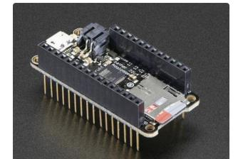
Finally, there's the "Stacking Header" option. This one is sort of the best-of-both-worlds. You get the ability to plug into a solderless breadboard and plug a featherwing on top. But its a little bulky
