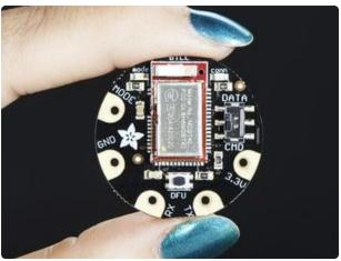
You can use this with just about any microcontroller with at least 3 pins, but best used with a Hardware Serial/UART capable chip!
