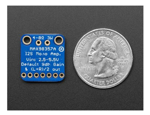
There's a Gain pin that can be manipulated to change the gain. By default, the amp will give you **9dB** of gain. By connecting a pullup or pull down resistor, or wiring directly, the Gain pin can be set up to give 3dB, 6dB, 9dB, 12dB or 15dB.
