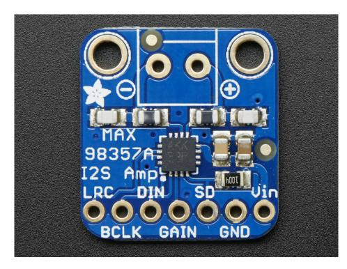
The MAX98357A is an **I2S** amplifier - it does not use analog inputs, it only has digital audio input support! Don't confuse I2S with I2C, I2S is a sound protocol whereas I2C is for small amounts of data.
