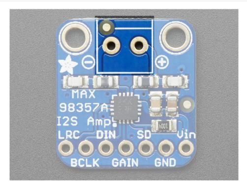
This amplifier is designed to drive moving coil loudpeakers only. Speaker impedence must be  $4\Omega$  or more. The
