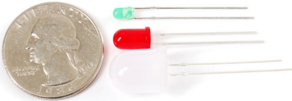
Green 3mm, Red 5mm and White 10mm LEDs
