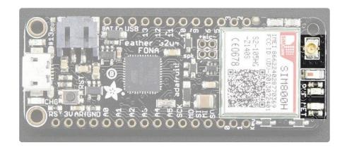
All the way to the right we have the cellular-only connection parts. Up top is a standard uFL connector, you attach your GSM antenna here
