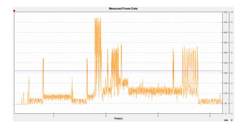
You can put the FONA into sleep mode (with the AT+CSCLK command) which will drop the current draw but keep the cellular connection open so you can still receive an SMS and/or wakeup quickly.
