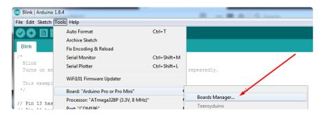
Once the Board Manager opens, click on the category drop down menu on the top left hand side of the window and select Contributed. You will then be able to select and install the boards supplied by the URLs added to the prefrences. In the example below, we are installing support for Adafruit AVR Boards, but the same applies to all boards installed with the Board Manager.
