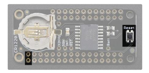
The Feather RESET pin is connected to a button on the right of the wing, handy if you need to reset or restart your Feather! Note that this RESET is not connected to the RS T pin on the DS3231
