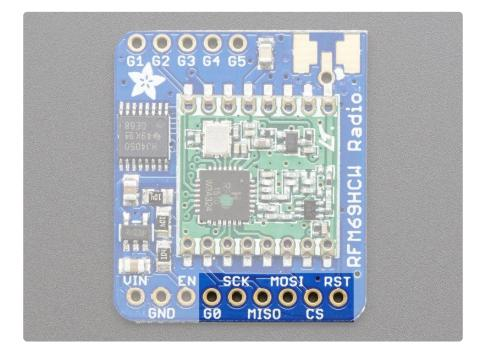
All pins going into the breakout have level shifting circuitry to make them 3-5V logic level safe. Use whatever logic level is on Vin!
