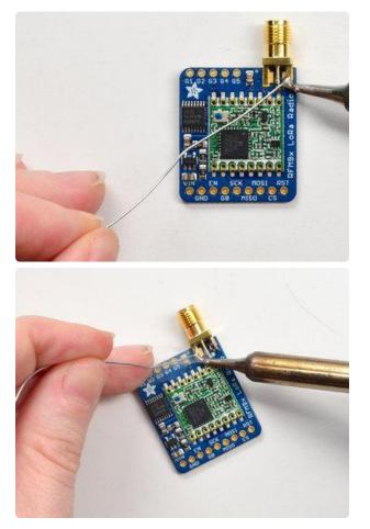
Solder in the two side ground pads. Note you will need a lot of heat for this, because the connector is an excellent heat sink and its got a huge ground plane
