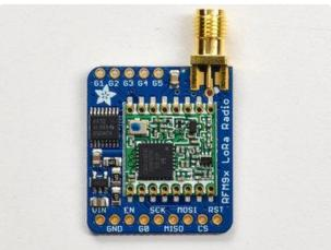
The SMA connector 'slides on' the top of the PCB
