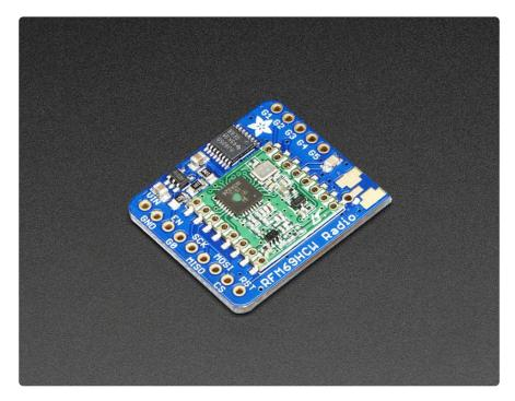
Also, these packet radios are simpler than WiFi or BLE, you don't have to associate, pair, scan, or worry about connections. All you do is send data whenever you like, and any other modules tuned to that same frequency (and, with the same encryption key) will receive. The receiver can then send a reply back. The modules do packetization, error correction and can also auto-retransmit so its not like you have to worry about e verything but less power is wasted on maintaining a link or pairing.
