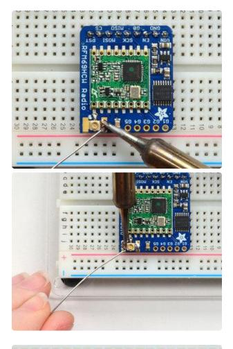
Solder in the two side pads, they are used for signal and mechanical connectivity so make sure there's plenty of solder
