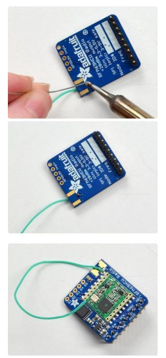
Strip a mm or two off the end of the wire, tin and solder into the ANT pad.
