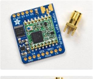
You'll need an SMA (or, if you need RP-SMA for some reason) Edge-Mount connector with 1.6mm spacing
