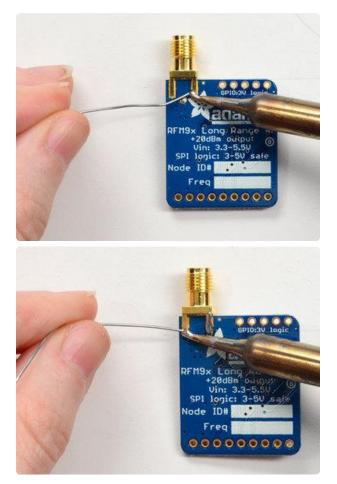
Flip over and also do the other side ground/mechanical contacts
