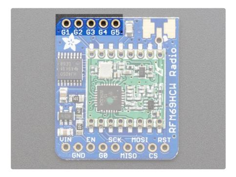
The radio's have another 5 GPIO pins that can be used for various notifications or radio functions. These aren't used for the majority of uses but are available in case you want them! All are 3.3V logic with no level shifting
