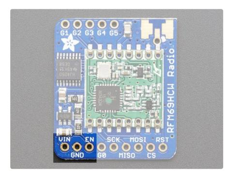
The left-most pins are used for power
