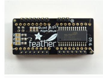
Flip over the kit and bend a few of the LED matrix legs out to keep the LED from slipping out while you solder
