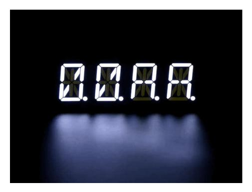
Upload to your Arduino, and open up the Serial console at 9600 baud speed. You'll see each digit light up all the segments, then the display will scroll through the 'font table' showing every character that it knows how to display. Finally, you'll get a notice to start typing into the serial console. Type a message and hit return, you'll see it scroll onto the display!
