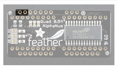
All LED control is done over I2C using the HT16K33 interface library. This means **SDA** (leftmost) and **SCL** (to the right of SDA) must be connected, see above for those pins.
