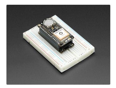
The Wing is built around the MTK3339 chipset, a no-nonsense, high-quality GPS module that can track up to 22 satellites on 66 channels, has an excellent high-sensitivity receiver (-165 dB tracking!), and a built in antenna. It can do up to 10 location updates a second for high speed, high sensitivity logging or tracking. Power usage is incredibly low, only 20 mA during navigation.
