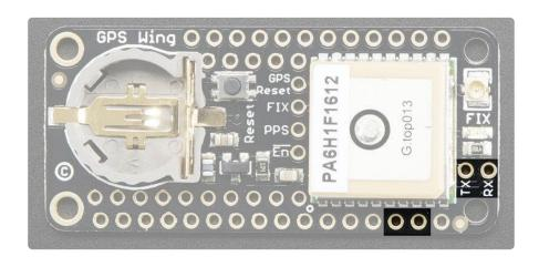
The GPS module, like pretty much all GPS's, communicates over UART serial. It sends ASCII NMEA setences from the GPS TX pin to the microcontroller RX pin and can be controlled to change its data output from the GPS RX pin. Logic level is 3.3V for both.
