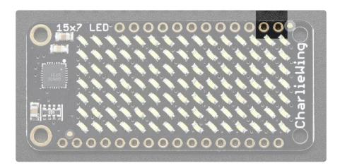
All LED control is done over I2C using the IS31FL3731 interface library. This means SD A (rightmost) and SCL (to the left of SDA) must be connected, see above for those pins.
