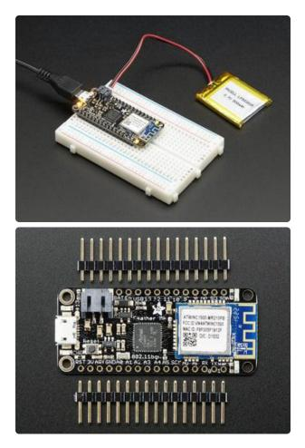
The first option is soldering in plain male headers, this lets you plug in the Feather into a solderless breadboard
