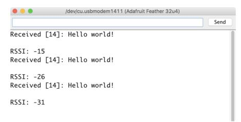
To receive a message simply call the **receive** function. This function will wait for half a second for any packet to be received. If a packet is found it will be returned as
