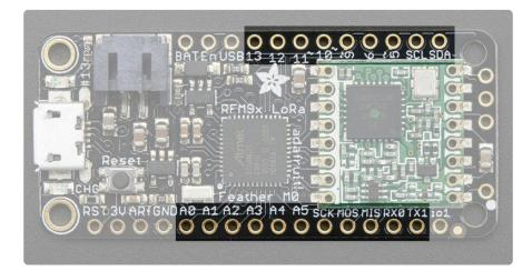
This is the general purpose I/O pin set for the microcontroller. All logic is 3.3V
