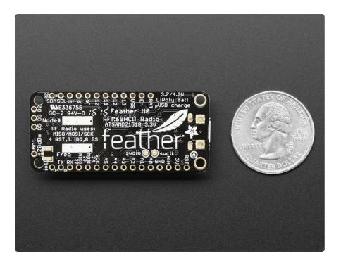
The Feather M0 Radio uses the extra space left over to add an RFM69HCW 433 or 868/915 MHz radio module. These radios are not good for transmitting audio or video, but they do work quite well for small data packet transmission when you ned more range than 2.4 GHz (BT, BLE, WiFi, ZigBee)
