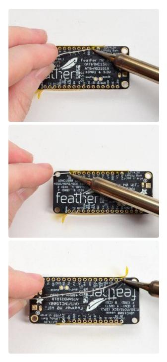
Flip & Tack Solder After flipping over, solder one or two points on each strip, to 'tack' the header in place
