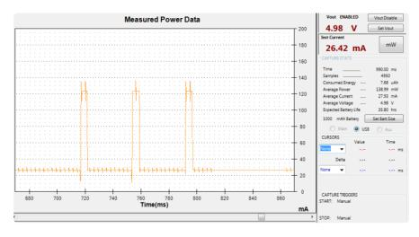
Here is a transmit with radio.setPowerLevel(0) to set +5dBm power
