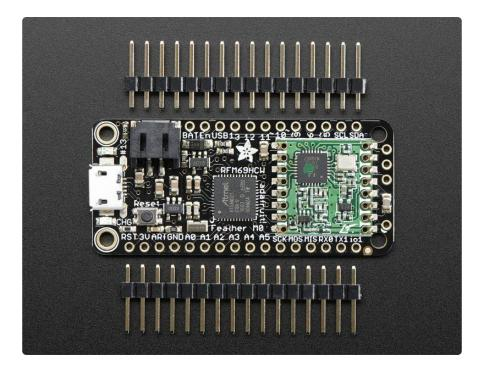
Comes fully assembled and tested, with a USB bootloader that lets you quickly use it with the Arduino IDE. We also toss in some header so you can solder it in and plug into a solderless breadboard. You will need to cut and solder on a small piece of wire (any solid or stranded core is fine) in order to create your antenna. Lipoly battery and USB cable not included but we do have lots of options in the shop if you'd like!
