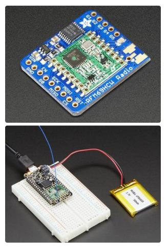
This page is shared between the RFM69 breakout and the all-in-one Feather RFM69's. The example code and overall functionality is the same, only the pinouts used may differ! Just make sure the example code is using the pins you have wired up.
