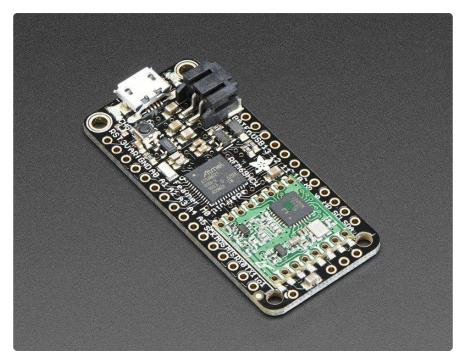
This is the Adafruit Feather M0 RFM69 Packet Radio (433 or 900 MHz) - our take on an microcontroller with a 433 or 868/915 MHz radio module cooked in! Great for making wireless networks that can go further than 2.4GHz 802.15.4 and similar, are more flexible than Bluetooth LE and without the high power requirements of WiFi. We have other boards in the Feather family, check'em out here (https://adafru.it/I7B)
