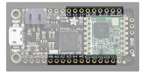
This is the general purpose I/O pin set for the microcontroller.
