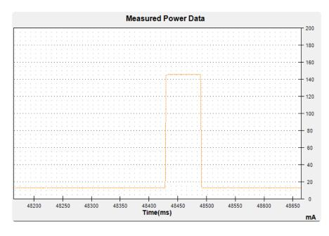
The ~13mA quiescent current is the current draw for listening (~2mA) plus ~11mA for the microcontroller. This can be reduce to amost nothing with proper sleep modes and not putting the module in active listen mode!
