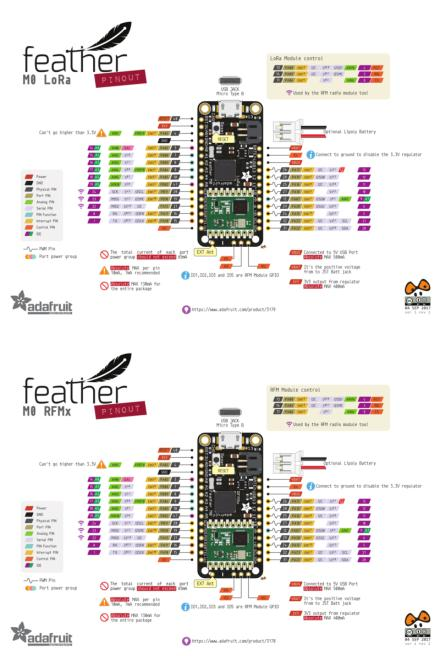
Note AREF in the diagram should be marked PA03 not PA02
