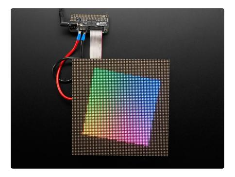
You can now create a dazzling display with your Raspberry Pi with the Adafruit RGB Matrix Bonnet. These boards plug into your Pi and makes it super easy to control RGB matrices such as those we stock in the shop and create a colorful scrolling display or mini LED wall with ease.
