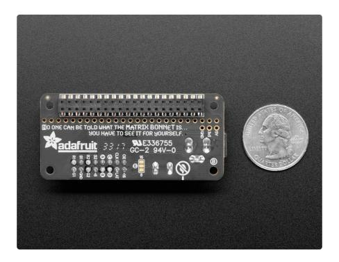
Works with any of our 16x32, 32x32 or 32x64 RGB LED Matrices with HUB75 connections (https://adafru.it/emd). You can also use 64x64 matrices by soldering a small jumper on the PCB (https://adafru.it/BhY). Want more lights? No problem, chain multiple matrices together for a longer display - we've only tested up to 32x128 but it works just fine. The bigger the display the harder it is on the Pi, so keep that in mind if you're using a lower-powered Pi Zero.
