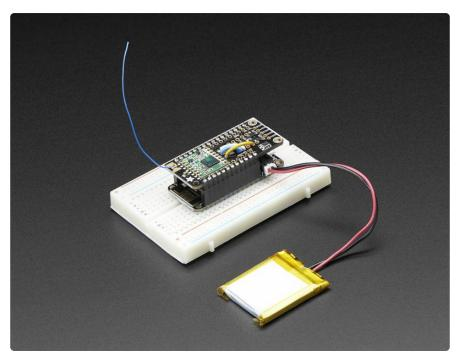
Add short-hop wireless to your Feather with these Radio Featherwings. These addons for any Feather board will let you integrate packetized radio (with the RFM69 radio) or LoRa radio (with the RFM9x's). These radios are good options for kilometerrange radio, and paired with one of our WiFi, cellular or Bluetooth Feathers, will let you bridge from 433/900 MHz to the Internet or your mobile device.
