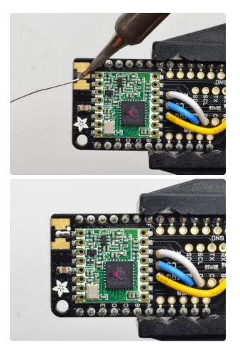
Start by melting solder onto the center signal pad
