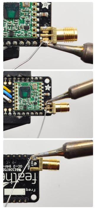
Solder all 5 connections (4 ground/ mechanical and 1 signal)
