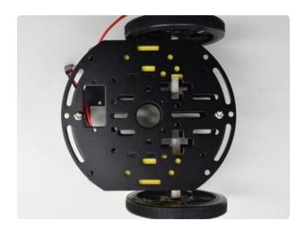
Place the next layer of the chassis on top of the motors. In this photo we didn't line up the second plate just like the first plate (note the off-set rectangle cut out) - this might fit for you or you might have to line them up with the same cutout to get a good fit
