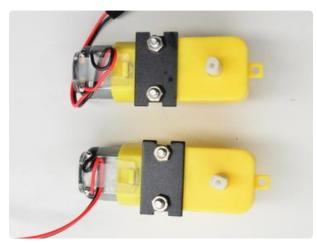
Screw the two black panels onto the motors. The metal panels go on the side with the red and black wires coming out
