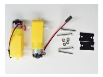
To start, take the two motors, four long screws, four nuts, and two black panels.
