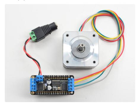
Stepper motors are great for (semi-)precise control, perfect for many robot and CNC projects. This motor shield supports up to 2 stepper motors. The library works identically for bi-polar and uni-polar motors
