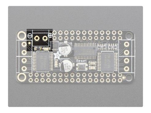
You must provide an external power supply for driving the motors. Provide 5-12V DC power + ground on these pins! Soldering in a terminal block will make it a little easier to swap in power supplies
