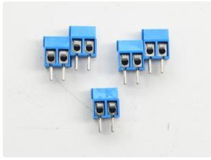
Next we will solder in the five 3.5mm terminal blocks used to connect power & the motors to the FeatherWing board.
