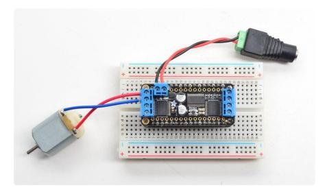
You must also supply 5-12VDC to power the motor. You can power the Wing via a connected DC Barrel Jack as seen above. A battery pack is good for portable use. Note that this will not power the Feather, that's normal - you want to keep separate power supplies and the Feather is best powered by a separate lipoly battery
