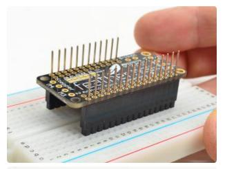
Flip it upside down so that the stacking headers fit over the headers in the breadboard
