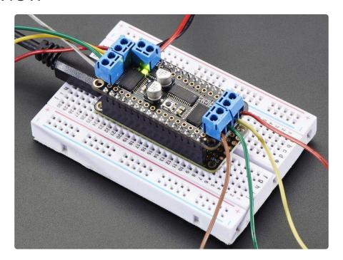
A Feather board without ambition is a Feather board without FeatherWings! This is the DC Motor + Stepper FeatherWing which will let you use 2 x bi-polar stepper motors or 4 x brushed DC motorx (or 1 stepper and 2 DC motors). Using our <u>Feather Stacking Headers</u> (http://adafru.it/2830) or <u>Feather Female Headers</u> (http://adafru.it/2886) you can connect a FeatherWing on top or bottom of your Feather board and let the board take flight!
