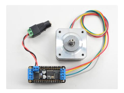
You must also supply 5-12VDC to power the motor. You can power the Wing via a connected DC Barrel Jack as seen above. A battery pack is good for portable use. Note that this will not power the Feather, that's normal - you want to keep separate power supplies and the Feather is best powered by a separate lipoly battery
