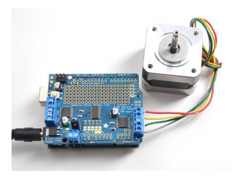
You must also supply 5-12VDC to power the motor. There are two ways to do this
