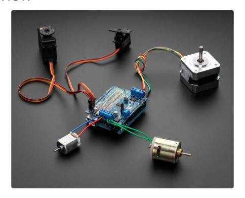
The original Adafruit Motorshield kit is one of our most beloved kits, which is why we decided to make something even better. We have upgraded the shield kit to make the bestest, easiest way to drive DC and Stepper motors. This shield will make quick work of your next robotics project! We kept the ability to drive up to 4 DC motors or 2 stepper motors, but added many improvements:
