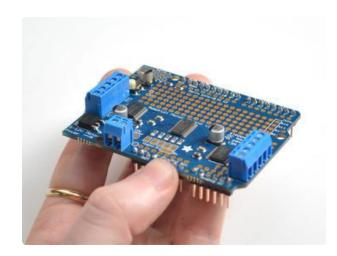
Next we will install the terminal blocks. These are how we will connect power and motors to the shield. They're much easier to use than soldering direct, just use a small screwdriver to release/attach wires!
