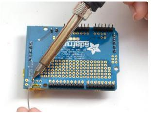
Then flip the board over and solder the 6 pins
