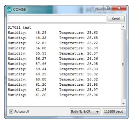
You can try breathing on the sensor to increase the humidity. The sensor reacts very fast!
