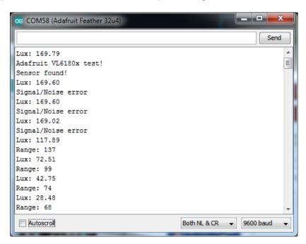
Move your hand up and down to read the sensor data, the range readings are in millimeters and the light sensors in Lux. Note that when nothing is detected, it will print out the error which may vary.
