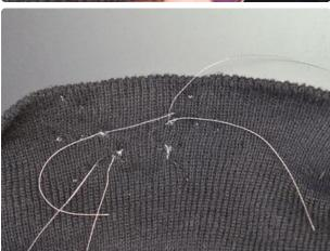
Next hook up the + connections from each of GEMMA's outputs to three pixels. We stitched from one sequin to the GEMMA, then over to another sequin and on to the third sequin before going back to the first, making a sort of square that results in the thread tails being in the same place.
