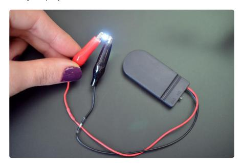
Simply connect 3 to 6VDC to the + pin and ground to the - pin, and the LED on the board will light up. In the photo above we've soldered alligator clips to a 2x2032 coincell battery holder ( $^{\sim}6V$ ). You could also use a single CR2032 sewable coincell holder-- you do not need a microcontroller to drive these sequins, unless you want them to blink or fade.
