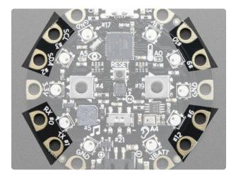
Of the 14 pads, you get a wide range of power pins, I2C, UART, Analog In, Digital In/Out and PWMt.
