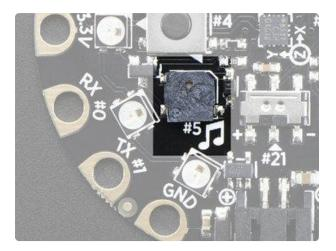
You can make your circuit playground sing with the built in buzzer. This is a miniature magnetic speaker connected to digital pin #5 with a transistor driver. You can use PWM at varying frequencies to make basic tones.
