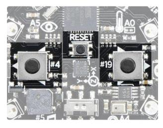
There are two large buttons, connected to digital #19 (Left) and #5 (Right) each. These are pulled to ground when not pressed, and connected to 3.3V when pressed, so they read HIGH.
