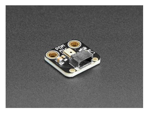
The first thing to note is that this sensor does not provide an 'analog' output like many of our electret microphone
