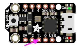
A0 is labeled "1 $^{\sim}$ " on Trinket! A0 is located between "0" and "2" towards the middle of the board on the same side as the red LED.
