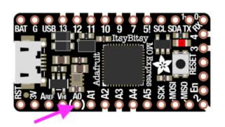
A0 is located between VHI and A1, near the "A" in "Adafruit", and the pin pad has left and right white parenthesis markings around it.
