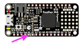
A0 is located between GND and A1 on the opposite side of the board from the battery connector, towards the end with the Reset button, and the pin pad has left and right white parenthesis markings around it
