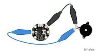
Use alligator clips to attach A2 and GND to different legs on the piezo.
