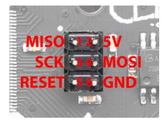
SCK/MOSI/MISO - These are the hardware SPI pins, are are connected to the 2x3 header on the right hand side. you can use them as everyday GPIO pins (but recommend keeping them free as they are best used for hardware SPI connections for high speed.)
