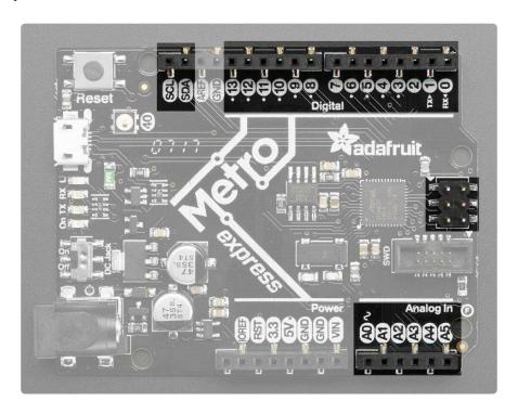
This is the general purpose I/O pin set for the microcontroller.
