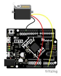
For the Metro M4 Express, ItsyBitsy M4 Express and the Feather M4 Express, connect the ground wire to any G or GND, the power wire to USB or 5V, and the signal wire to A2.
