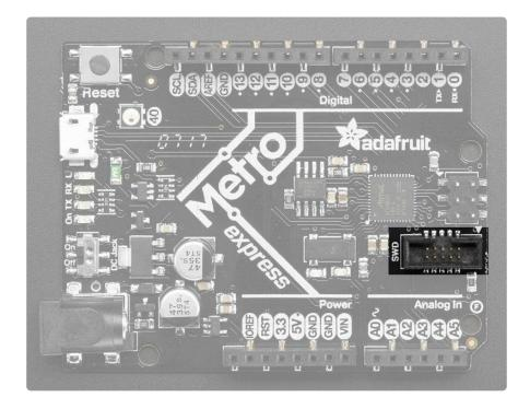
If you'd like to do more advanced development, trace-debugging, or not use the bootloader, we have the SWD interface exposed.
