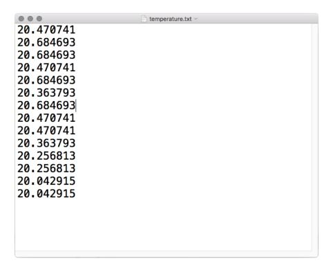
This file gets updated once per second, but you won't see data come in live. Instead, when you're ready to grab the data, eject and unplug your board. For CPX, move the switch to the left, otherwise remove the wire connecting the pin to ground. Now it will be possible for you to write to the filesystem from your computer again, but it will not be logging data.
