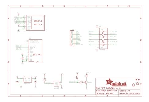
For the level shifter we use the  $\underline{\text{CD74HC4050}}$  (https://adafru.it/CgA) which has a typical propagation delay of ~10ns
