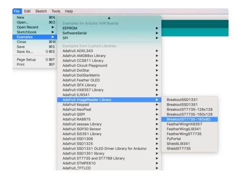
Now upload the example sketch to the Arduino. You should see ADABOT appear! If you have any problems, check the serial console for any messages such as not being able to initialize the microSD card or not finding the image.
