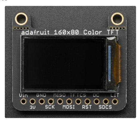
This color display uses SPI to receive image data. That means you need at least 4 pins - clock, data in, tft cs and d/c. If you'd like to have SD card usage too, add
