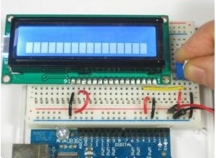
This means you've got the logic, backlight and contrast all worked out. Don't keep going unless you've got this figured out!
