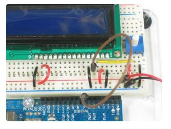
Next is the RS pin #4. We'll use a brown wire to connect it to Arduino's digital pin #7.
