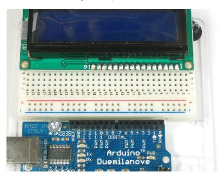
The easiest way we know of doing this is sticking the header into a breadboard and then sitting the LCD on top while soldering. this keeps it steady.
