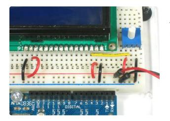
Now we'll wire up the logic of the LCD - this is seperate from the backlight! Pin 1 is ground and pin 2 is +5V.
