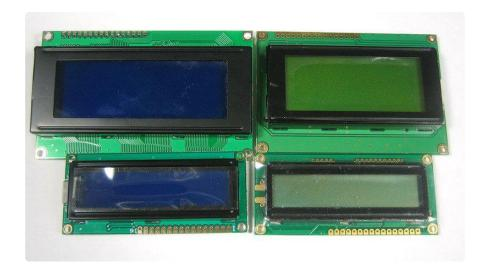
Although they display only text, they do come in many shapes: from top left we have a 20x4 with white text on blue background, a 16x4 with black text on green, 16x2 with white text on blue and a 16x1 with black text on gray.
