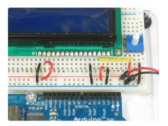
As mentioned, we'll not be using the RW pin, so we can tie it go ground. That's pin 5 as shown here.
