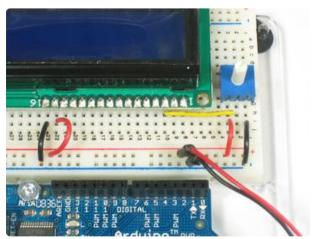
Connect one side of the pot to +5V and the other to Ground (it doesn't matter which goes on what side). The middle of the pot (wiper) connects to pin 3 of the LCD.
