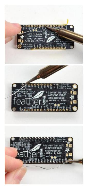
And Solder! Be sure to solder all pins for reliable electrical contact.
