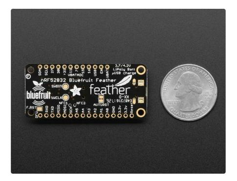
The Adafruit Feather nRF52 Pro ships pre-programmed with the Mynewt serial bootloader that allows you to flash firmware to the device directly from the commandline using the on-board USB Serial converter and the 'newtmgr' tool, so you can get started right away with no additional hardware required. For more advanced debugging, however, you can use a Segger J-Link and the on-board SWD debug connector, which gives you access to a more powerful set of development tools and options.
