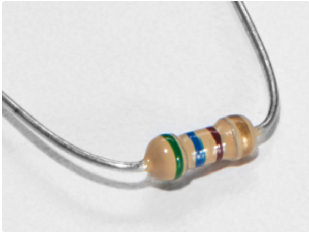
560 Ohm Resistor Colors: Green > Blue > Brown
