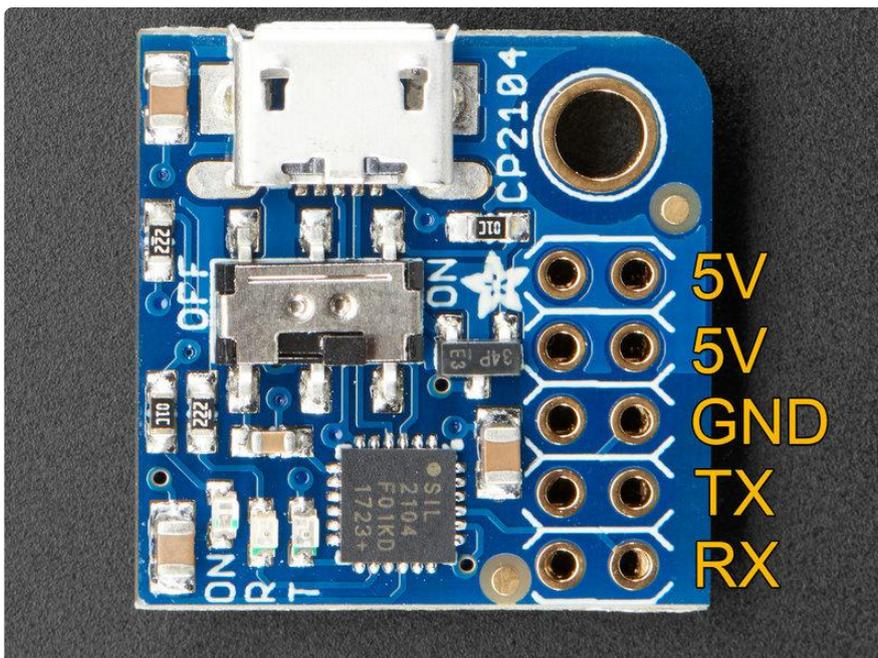
We only use the 'right' strip of the dual header but to make it more mechanically stable we have a dual header to plug into.
