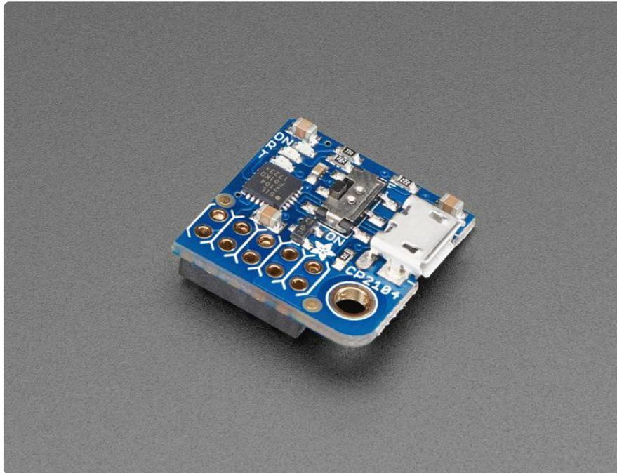
Here's another super handy add-on for your Raspberry Pi computer, perfect for 'head-less' setups! The [PiUART](https://adafruit.it/zib) (<https://adafruit.it/zib>) adds a MicroUSB to serial connection so you can use any serial port software to connect to the Pi's console. It plugs in and is fast and easy to add whenever you need to connect to your Pi. Two LEDs connect to RX and TX on the serial converter chip so you get blinking whenever data is sent or received.
