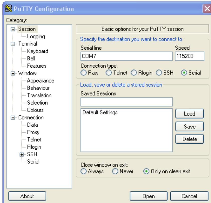
Select a connection type of "Serial" from the radio buttons, then set the speed to 115200 and the serial line to COM7
