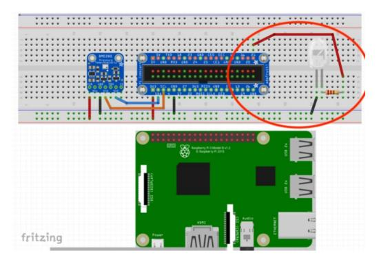
The included 560 Ohm and 10K Ohm resistors will both protect the circuit, the latter make the LED dim. You can sanity check your wiring with python using the following commands one by one:
