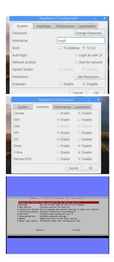
3. Once rebooted and connected to a network we can secure shell into our Pi remotely or use the command line directly to update our Linux distro and Raspberry Pi 3 firmware. The default uersname is "pi", default password is "raspberry ". To get the Pi's IP, use the command "ifconfig" or nmap your subnet for new ssh services. However you connect, update your Pi with the following commands and change your pi's default password with the "passwd" command if you so choose.
