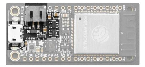
The above shows the Micro USB jack (left), Lipoly JST jack (top left), as well as the 3.3V regulator (to the right of the JST jack), changeover diode+transistor (below the JST jack) and the Lipoly charging circuitry (right below the regulator).
