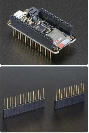
Finally, there's the "Stacking Header" option. This one is sort of the best-ofboth-worlds. You get the ability to plug into a solderless breadboard and plug a featherwing on top. But its a little bulky
