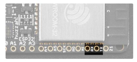
The TX pin is the output from the module. The RX pin is the input into the module. Both are 3.3V logic
