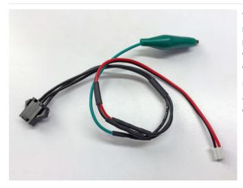
To connect the microcontroller at the "input" end of the strand, I soldered up this little **adapter cable** using a **3pin JST plug** (to the LEDs), a **2-pin JST cable** (to the Circuit Playground, Flora or Gemma board) and one end of an **alligator jumper cable**.
