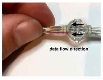
NeoPixel color data must travel from the "in" end of the strand to the "out" end. Examine the backs of the pixels *very* closely. Printed on the PCB, you might see either some data direction arrows, or the words "IN" and "OUT" between pads. The weatherproofing epoxy makes things murky and you may need to look at several pixels before finding one. This is important! If you connect the microcontroller to the wrong end, the lights won't work.
