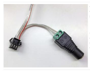
Connect a female DC power adapter using the screw connectors, being **super extra careful** to **follow the polarity markings** stamped on the DC jack:
