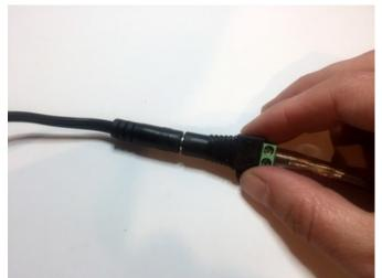
**Double-check** all your connections: 5V, ground and NeoPixel data. If you have a multimeter with a continuity beep function, the "–" (minus) terminal on the DC jack should beep in response to any "GND" pad on the microcontroller board.
