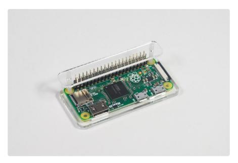
Using a hammer, gently tap back and forth on the top acrylic piece to push the pins through. Pushing one end of the header all the way it can cause the other pins to bend when you hammer them in. It's worth taking your time over this part.
