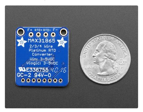
We've carried various MAXIM thermocouple amplifiers and they're great - but thermocouples don't have the best accuracy or precision, for when the readings must be as good as can be. The MAX31865 handles all of your RTD needs, and can even compensate 3 or 4 wire RTDs for better accuracy. Connect to it with any
