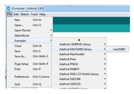
Upload to your Arduino and open up the serial console at 115200 baud to see a print out of the sensors data. The MAX31865 doesn't actually return the resistance it measures. Instead it returns the ratio between the resistance measured and the Rref reference resistor.
