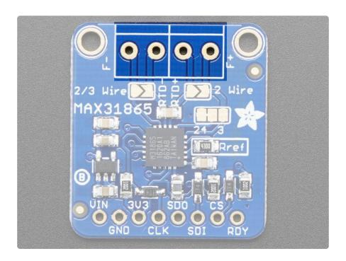
If you have an RTD sensor, you need to connect it somehow! the terminal block area is where you can clamp down to the sensor wires.
