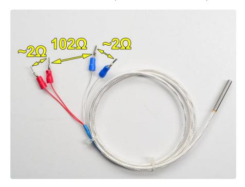
(Remember that the middle resistance - 102 or 1002  $\Omega$  - will vary with temperature, but the  $2\Omega$  wires will not) When the amp measures this sensor, it will measure the resistance between one set of red and blue wires. It will then measure the resistances between the red wires and blue wires. Then divide those resistances by half - since there's two wires and we just want the resistance of one wire. The final result is 102 - 1 - 1 =  $100\Omega$
