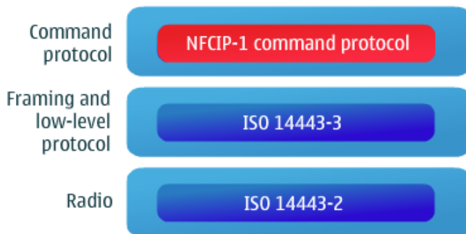
Figure 6: ISO 14443 protocol stack
