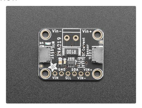
The INA219B breakout board and the INA219 FeatherWing will solve all your power-monitoring problems. Instead of struggling with two multimeters, you can use this breakout to measure both the high side voltage and DC current draw over I2C with 1% precision.
