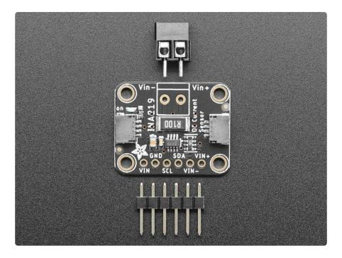
As if that weren't enough, we've now also added <u>SparkFun qwiic</u> (https://adafru.it/Fpw) compatible <u>STEMMA QT</u> (https://adafru.it/Ft4) connectors for the I2C bus so you don't even need to solder the I2C and power lines. Just wire up to your favorite micro
