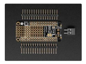
Solder the headers and the screw terminal to the board in the appropriate locations.
