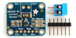
The board comes with all surface-mount components pre-soldered. Additional parts are included to help integrate the INA219 breakout board into your project.
