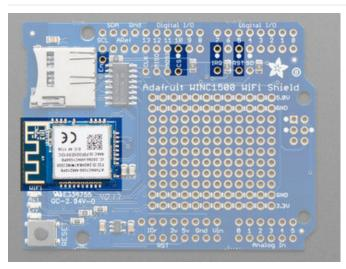
The WiFi module is where the magic happens. In addition to the SPI pins, the WINC module also requires three GPIO for control:
