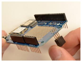
Insert the 2x3 stacking header as shown.
