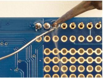
Once you've tacked and straightened all the headers, go back and solder the remaining pins for each header.
