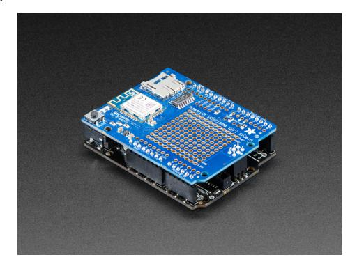
Connect your Arduino-compatible to the Internet with this WiFi shield that features the FCC-certified ATWINC1500 module from Atmel. This 802.11bgn-capable WiFi module is the best new thing for networking your devices, with SSL support and rock solid performance - running our adafruit.io MQTT demo for a full weekend straight with no hiccups (it would have run longer but we had to go to work, so we unplugged it).
