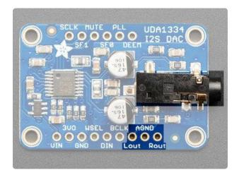
The exciting part! This is where your line level audio comes out. We put big 47uF blocking capacitors on the output so you can connect this to any stereo system. AGND is a clean analog ground signal that we recommend using as your analog reference, you'll get a cleaner signal.
