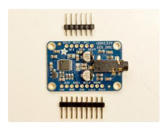
Break apart the 0.1" header into 6 and 9pin long pieces and slip the short ends into the holes in the board
