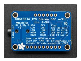
SFO and SF1 are used to set the input data format. By default both are pulled Low for I2S but you can change them around for alternate formats.
