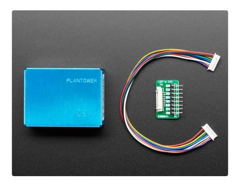
You'll need to hook this up to a microcontroller with UART input (or you could theoretically wire it up to a USB-Serial converter and parse the data on a computer (https://adafru.it/C7B)) - we have code for both Arduino and CircuitPython. 9600 baud data streams out once per second, you'll get:
