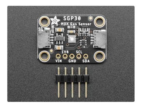
The SGP30 has a 'standard' hot-plate MOX sensor, as well as a small microcontroller that controls power to the plate, reads the analog voltage, tracks the baseline calibration, calclustes TVOC and eCO2 values, and provides an I2C interface to read from. Unlike the CCS811, this sensor does not require I2C clock stretching.
