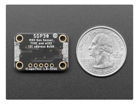
This part will measure eCO2 (equivalent calculated carbon-dioxide) concentration within a range of 400 to 60,000 parts per million (ppm), and TVOC (Total Volatile Organic Compound) concentration within a range of 0 to 60,000 parts per billion (ppb).
