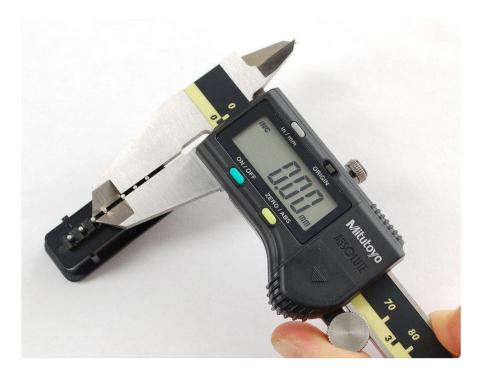
Now you can measure on the outer edges of the pins and it will automatically subtract one pin thickness.
