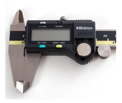
Digital calipers do require a battery (there are solar ones as well, with an internal backup battery) but good calipers rarely need to have the battery replaced. The pair we have is used many times a day and often isn't even turned off for a few days but
