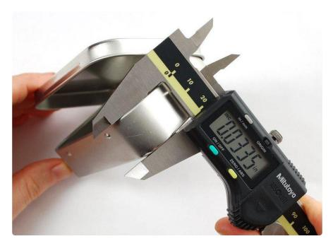
This measurement came out to 33.5 mils. <u>The closest standard sheet gauge</u> (https:// adafru.it/aJ8) to 0.0335 is 20 gauge. Variations in the metal thickness may be due to additional thickness from the plating process or the rounded edges interfering with the depth measurement. Taking multiple measurements is always a good idea!
