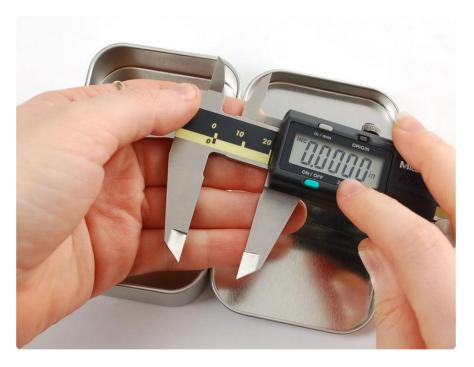
And measure the overall thickness. The difference is the thickness of the bottom metal.
