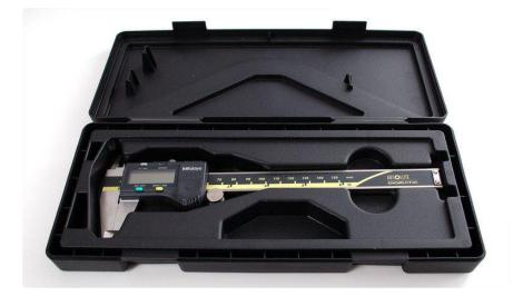
Keep your calipers happy and safe in their box. Even though digital calipers are in many ways more durable than mechanical/dial types, especially with respect to shock, when traveling or storing, keep 'em in the case!
