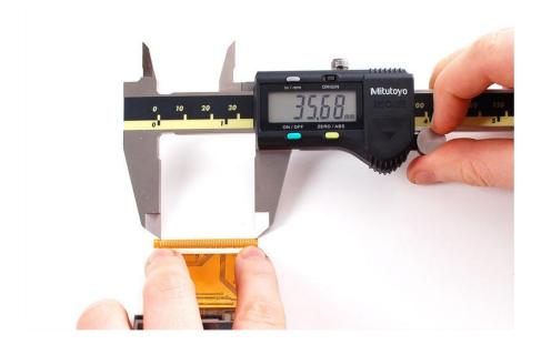
Remember that for a N pin connector, there are N-1 'gaps' (a common-enough confusion that it has its own name, the <u>fencepost-error</u> (https://adafru.it/aJ9) ) so divide 35.68mm by 36 = 0.99mm. Since we're eyeballing the center points of the connector, this should be rounded up to a 1mm pitch. Sometimes the number should be rounded up/down in imperial so if it seems off, check other units.
