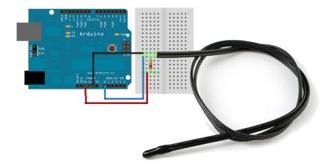
Connect one end of the 10K resistor to 5V, connect the other end of the 10K 1% resistor to one pin of the thermistor and the other pin of the thermistor to ground. Then connect Analog 0 pin to the 'center' of the two.
