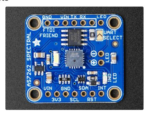
This sensor has 4 mounting holes and 2 header breakout strips.
