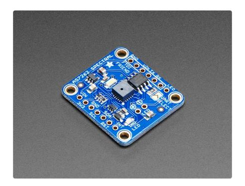
The 6 channels on the AS7262 are realized by silicon interference filters at 450nm, 500nm, 550nm, 570nm, 600nm, and 650nm. This breakout uses the I2C interface on the chip by default, but a UART interface that accepts AT commands is also selectable.
