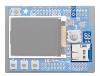
The micro SD card slot can be used to read/write data from any micro SD card using the Arduino libraries. The SD card is connected to the SPI pins as well as Digital #4 for Chip Select
