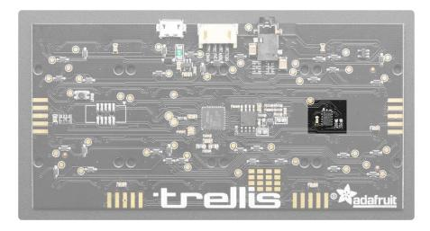
This sensor is on a separate I2C port, which is available in Arduino under Wire1 or in CircuitPython under <a href="mailto:board.ACCELEROMETER\_SCL">board.ACCELEROMETER\_SDA</a>
