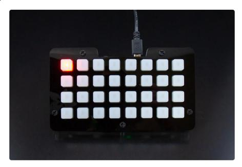
The TrellisM4 library has the ability to specify four different orientations in 90 degree increments by setting rotation in the setup line equal to: 0, 90, 180, or 270. This allows you to rotate your board with ease to the position that works best for your project, without requiring complicated code to compensate. We do that for you! The coordinates of the buttons change with the rotation, so (0, 0) is always top-left. Let's look at some examples.
