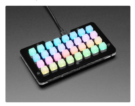
The NeoTrellis M4 is an all-in-one USB + NeoPixel + Elastomer + Audio board. It's powered by our new favoritest-chip-in-the-world, the SAMD51, a Cortex M4 core running at 120 MHz. This chip has a speedy core with CircuitPython and Arduino support, hardware DSP/floating point, dual DACs (more on that later!) and all the
