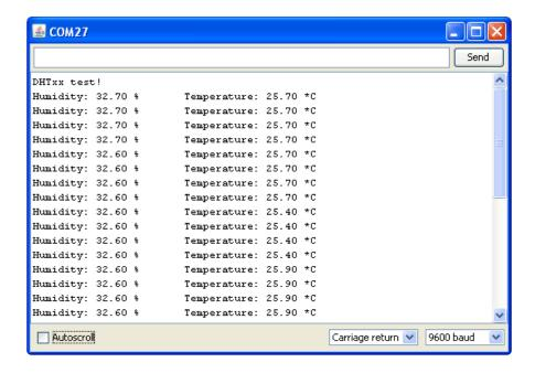
You should see the temperature and humidity. You can see changes by breathing onto the sensor (like you would to fog up a window) which should increase the humidity.
