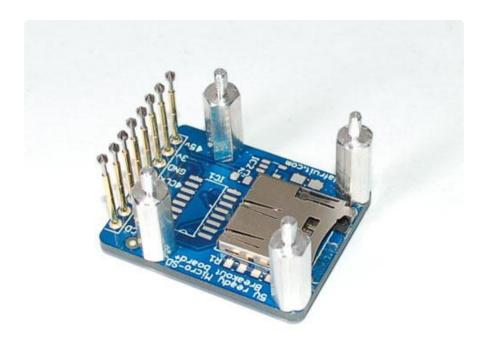
Choose the standoffs so that the tips of the pogo pins are above the standoff part but below the end of the screw.
