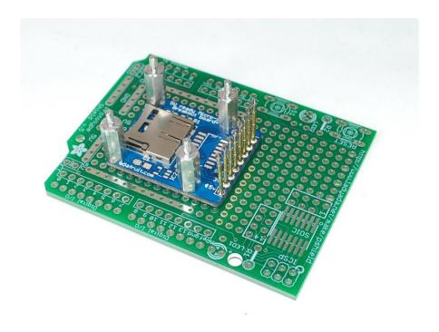
Mark and drill the mounting holes - four in this case. Luckily (or on purpose???) I placed the mounting holes on 0.1" boundaries.
