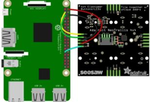
Wiring is easy, solder the four VIN GND SDA SCL pads to wires and then connect to your CircuitPython device
