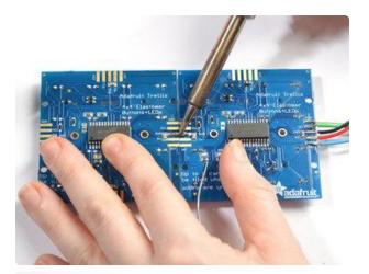
Use your soldering iron to drag solder from one pad to another, with a little effort they'll stick together and make a connection. You can add more solder to make the connection stronger. Its still not mechanically strong - so be careful not to bend or shake the arrangement
