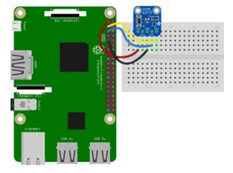
Here's the Raspberry Pi wired with I2C:
