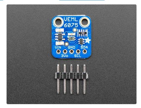
Each order comes with one assembled PCB with a sensor, power regulator, level shifting and a small piece of header. Some light soldering is required to attach the header but its a fast task!
