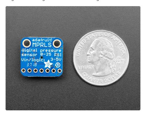
We've placed this nice sensor on a breakout board with 3.3V power regulation and level shifting so you can use it with any kind of microcontroller or microcomputer, from an Arduino compatible to Raspberry Pi
