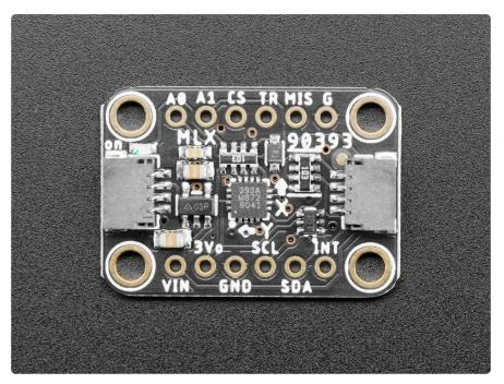
Measure the invisible magnetic fields that surround us, with this wide-range magnetometer. The MLX90393 is a wide range magnetic field sensor, that can measure 16-bits in ranges from +/-5mT up to +/-50mT in all 3 axes.
