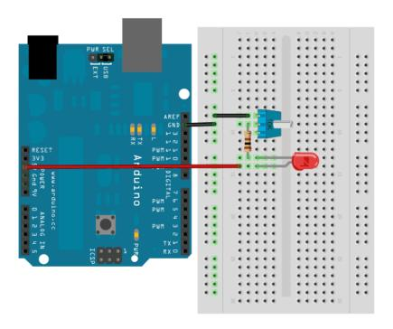
Note that we are connecting to the wiper and one end, not to both ends. Also, we have a 100 ohm resistor between the potentiometer and the LED.
