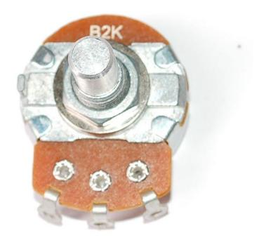
Potentiometers, like resistors, have an Ohm value. For example, this potetiometer is a 2Kohm (its printed up top). Potentiometers have three pins, two 'outer' and one 'middle' pin. The middle pin is sometimes called the wiper.
